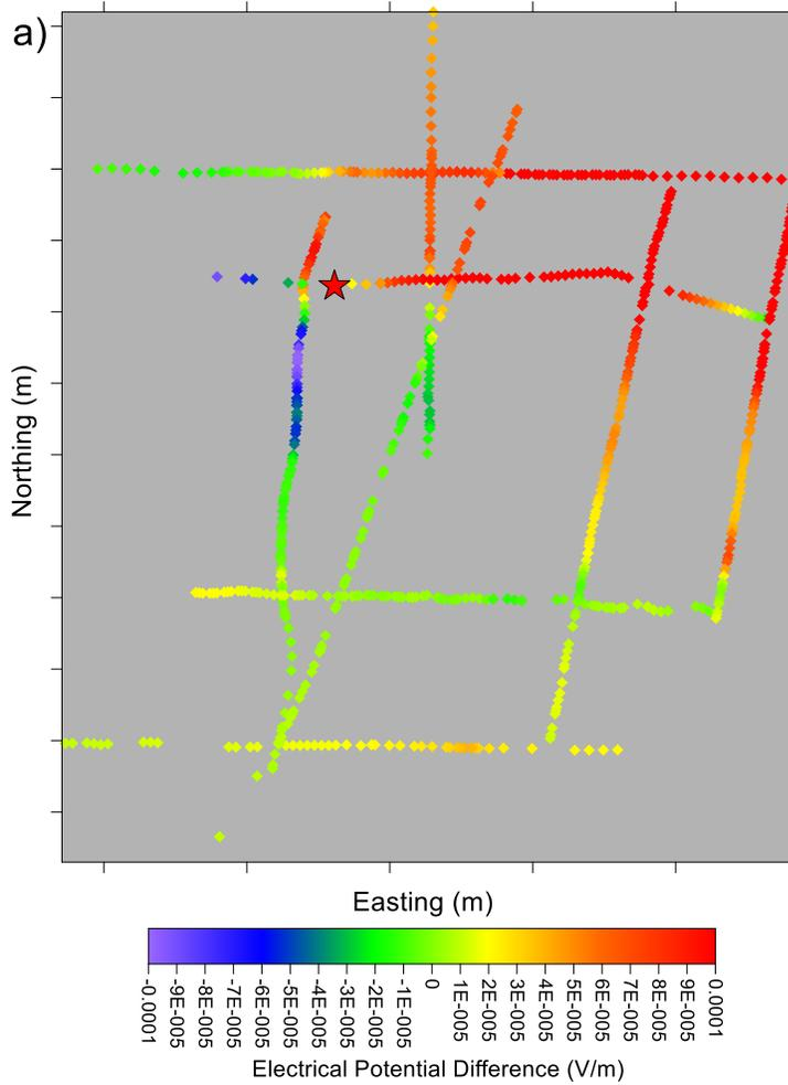
**Figure 7: Raw potential differences. For typical MALM surveys this data would be used directly to interpret the limits of the subsurface conductive body. The atypical survey geometry made the usual interpretation for this dataset difficult without further processing**
