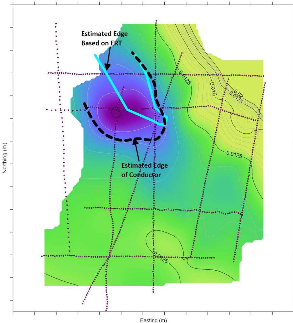
**Figure 8: Processed potential difference surface. The limit of the conductive aquifer based on the MALM is indicated by the dashed black line. The limit of the conductive aquifer based on the ERT is indicated by the cyan line. The difference between the two limits is likely due to the limitations of the ERT when the aquifer becomes very thin.**
