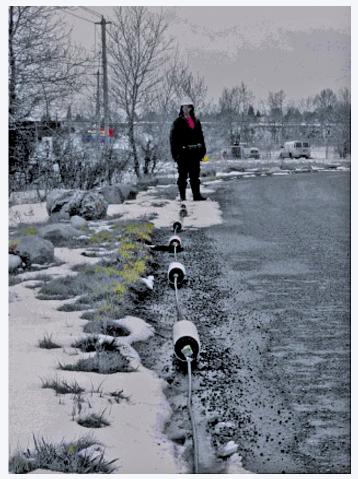
Figure 3. Towed OhmMapper array.
