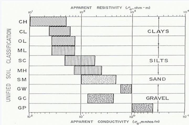
Figure 2. Resistivity ranges of soil as defined by the Unified Soil Classification scheme (adapted from Kaufman and Hoekstra, 2001) Resistivity is the inverse of conductivity.
