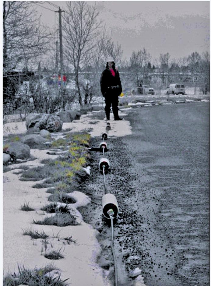
Figure 3. Towed OhmMapper array.
