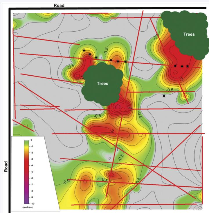
Figure 6. Depth to the base of interpreted aggregate material. Survey lines are in red. Colour scale grades from grey, representing minimum depth (i.e. surface) to purple, representing maximum depth of aggregates. Contour interval is 0.5 metre.
