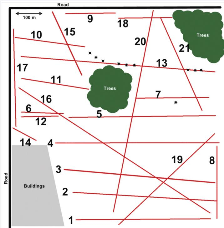
Figure 1. Site map showing OhmMapper survey lines (red) and test pit (black asterisk) locations.
