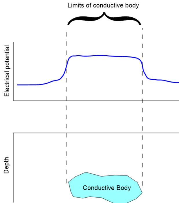
**Figure 4: Illustration of the electrical potential over a conductive body for a typical MALM survey. The limits of the conductive body are determined based on the potential drop-off at its edges.**
