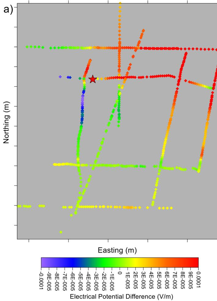
**Figure 7: Raw potential differences. For typical MALM surveys this data would be used directly to interpret the limits of the subsurface conductive body. The atypical survey geometry made the usual interpretation for this dataset difficult without further processing**
